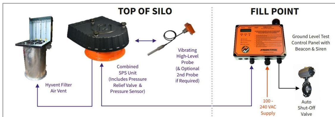
A successful 6 second test of the complete system opens the failsafe fill point valve to allow filling for 90 minutes after which it will close. A siren and beacon will also sound to test their operation.
