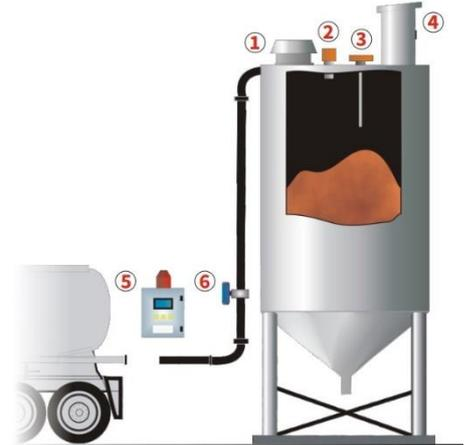
The SHIELD Lite silo protection system is designed to provide control and test functions to prevent silo over-pressurisation and filter blinding during a tanker delivery. The system can work with one or two level probes of different lengths; these can be Hycontrol level probes which have a built-in GLT (Ground Level Testing). It is simple to install, can be retro-fitted to existing tank silos and is easy to operate.
